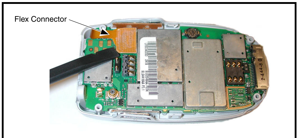
Figure 8. Disconnecting the flex from the transceiver board
