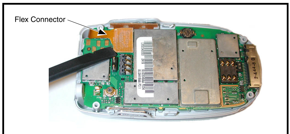
Figure 8. Disconnecting the flex from the transceiver board
